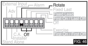
The Fixed Last / Off DIP switch selects whether or not the last boiler is to be included in the rotation sequence. If the DIP switch is set to Fixed Last, the last boiler is always the last to fire (FIG. 47). This DIP switch is only active when the Rotate / Off DIP switch is set to Rotate. FIXED LEAD / OFF
